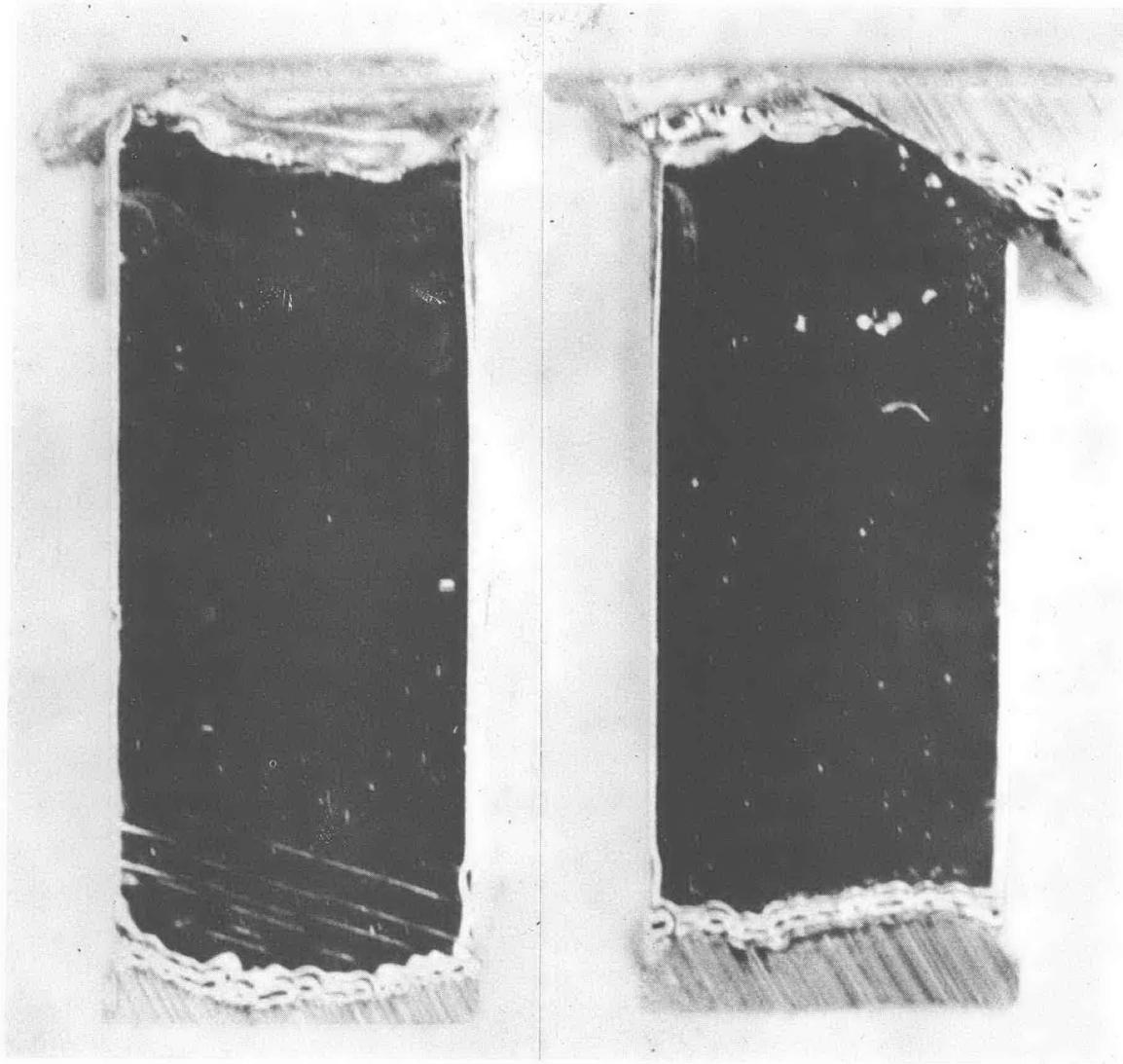
Fig. 8 - Macroscopic Photograph Showing  $\{11\bar{2}0\}$  and  $\{10\bar{1}0\}$  Lateral Surfaces of Crystal ISR-11 After c-axis Compression under Hydrostatic Pressure in the Range 238-255 ksi. Mag. 15X
